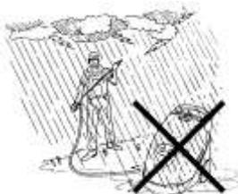
Please, protect the machine from atmospheric agents. Avoid using the machine under the rain or thunderstorms, and in all situations when water or other liquids can reach the electrical parts.
