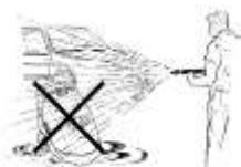
It is forbidden to direct the water jet onto the pump and, anyway, onto any other object under electric tension. This can cause electrical damage and danger for the user.
