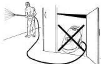
Do not use the machine in closed rooms, nor where the ventilation is inadequate.
