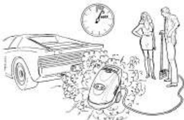
Do not leave the machine on with the gun closed for more than five minutes. Beyond this limit the pump becomes overheated, getting damaged and endangering the user. (Only for machines without Totalstop).
