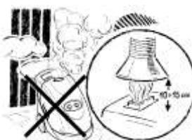
Install a device for discharging combustion gases into the atmosphere. Discharging combustion gases inside closed premises is highly dangerous!
